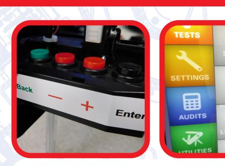
Use buttons inside coin door to access & navigate Test Menu.
